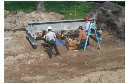
Compression load test
