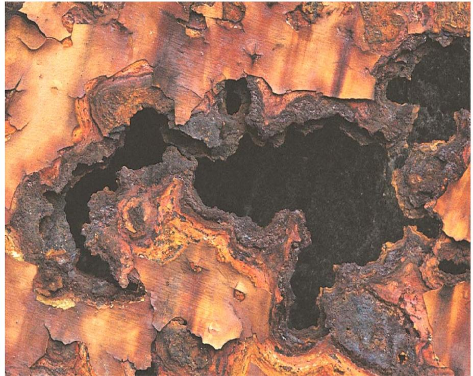
**The Rate of Corrosion** is heavily influenced by the nature of the soil
