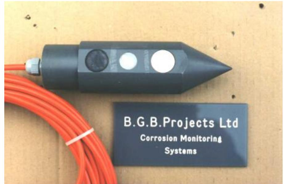
**Corrosion Rate** testing using linear polarisation testing (LPR) method at 1.5m, 4m, and 8m depths
