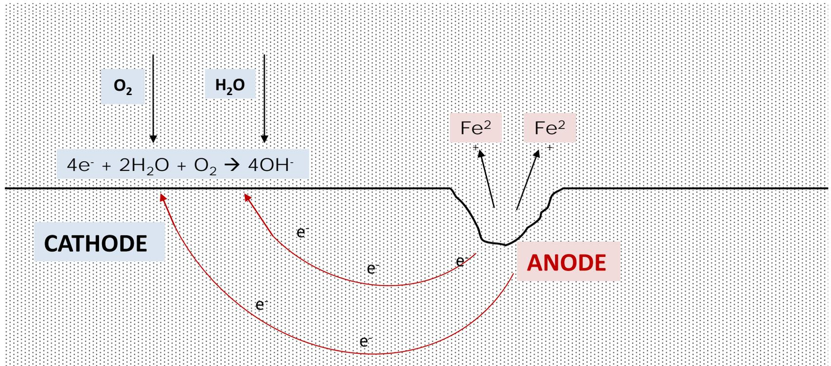
**Corrosion** As the electrochemical reaction takes place, differences in the surface potential also changes with time and the **ANODE** can move to another location, one that may even have previously been a **CATHODE**. The result therefore is an appearance of all-over '**GENERAL CORROSION**'.
