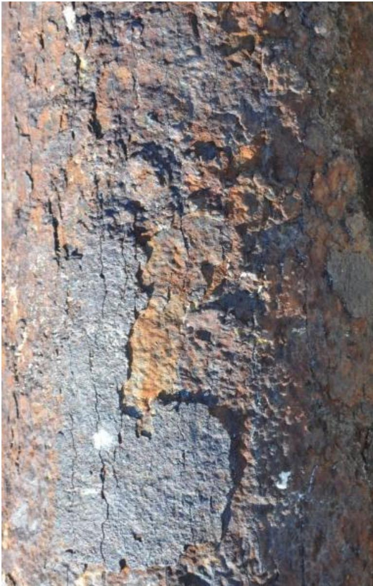
A metal surface will have discrete areas with differences in potential caused by variations in surface characteristics, inclusions, moisture or from being embedded in variable soils.
