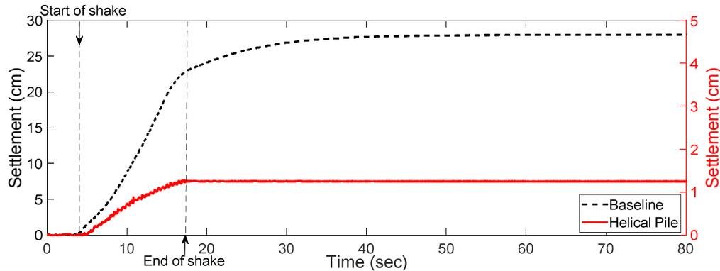
**Fig. 9. Foundation settlement during baseline and helical pile tests.**
