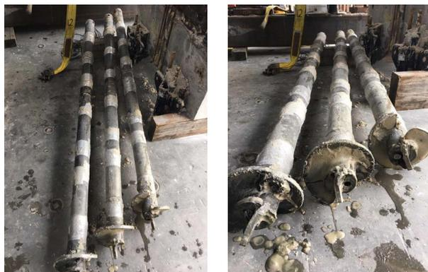
**Fig. 6. Extracted helical piles after test completion.**
