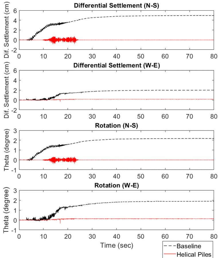
**Fig. 8. In-plane and out-of-plane rotation and differential settlement for baseline and helical pile tests.**
