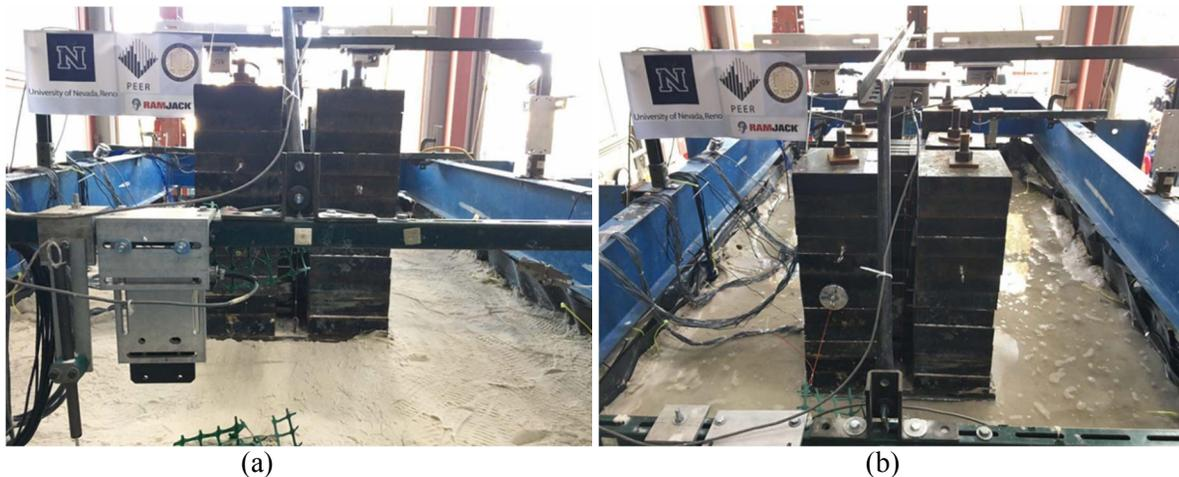
**Fig. 5. Model shallow foundation (a) before and (b) after completion of helical pile test.**
