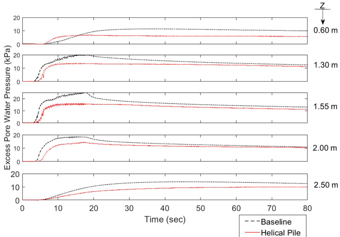
**Fig. 7. Excess pore water pressure generation along depth during baseline and helical pile tests for below foundation array of sensors.**
