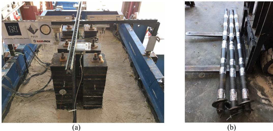
**Fig. 2. (a) Model shallow foundation configuration for helical pile test before shaking, (b) Helical piles configuration after instrumentation (Helical piles provided by Ram Jack).**
