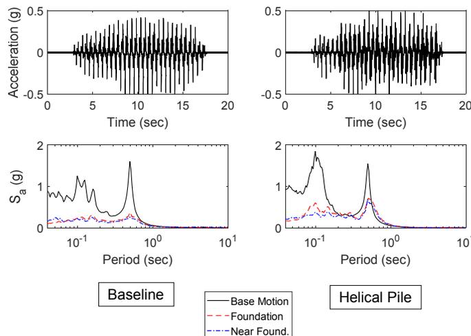
**Fig. 4. Recorded motion characteristics in baseline and helical pile tests.**
