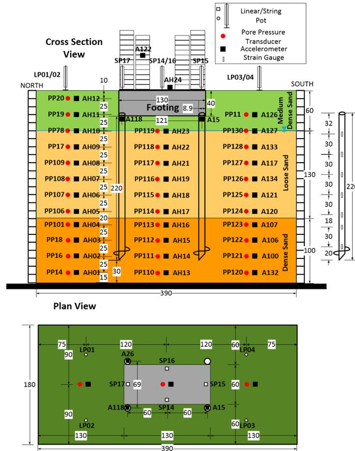
**Fig. 3. Model configuration and instrumentation plan for helical pile test (All dimensions are in centimeters).**
