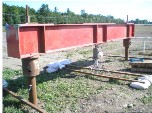
Figure 2. Typical axial compression test setup
