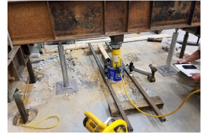
Helicast pile load test
