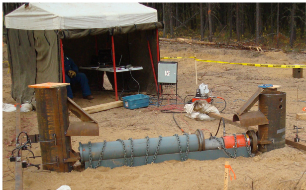
Figure 3. Typical lateral load test setup
