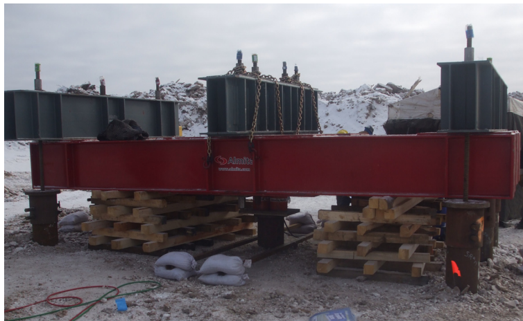
Fig. 3. Typical axial compression test setup
