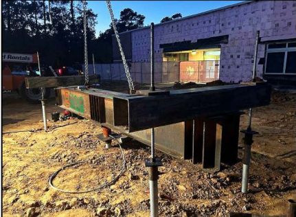
Set Up for A.M. Load Test
