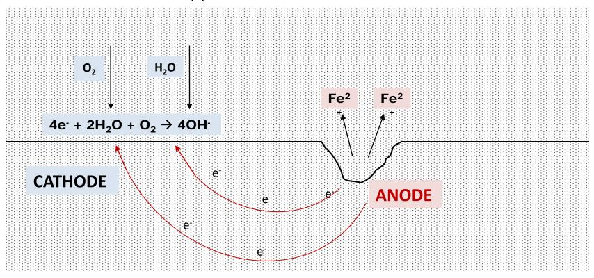
**Corrosion** As the electrochemical reaction takes place, differences in the surface potential also changes with time and the **ANODE** can move to another location, one that may even have previously been a **CATHODE**. The result therefore is an appearance of all-over 'GENERAL CORROSION'.
