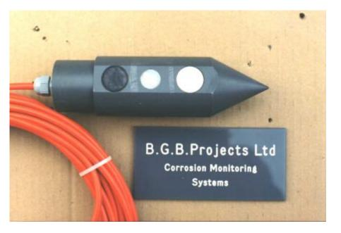
**Corrosion Rate** testing using linear polarisation testing (LPR) method at 1.5m, 4m, and 8m depths
