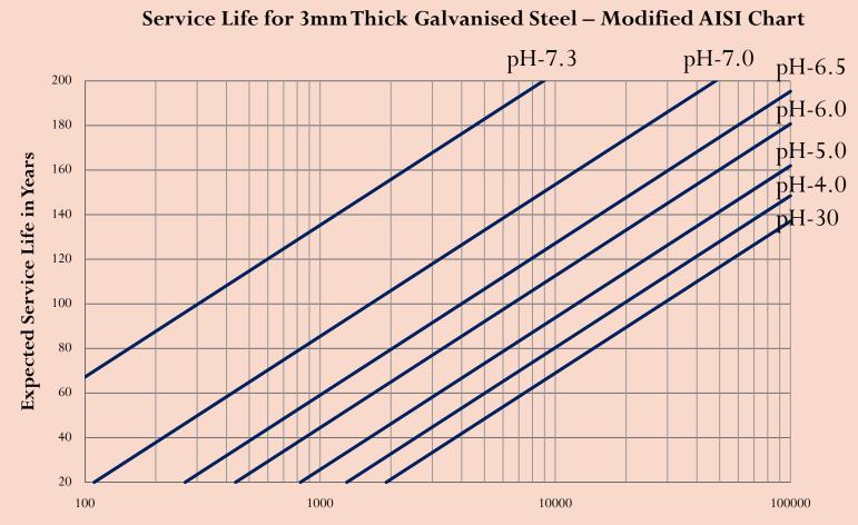
Soil Resistivity (R) in Ohm.cm - Service Life = 1.9 x 35.85 x (log R - log(2160-2490 x log(pH)))
