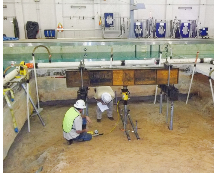
Compression load test
