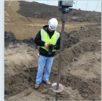
Helical test probe; torque monitored with calibrated torque transducer
