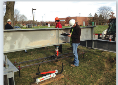
Compression load test
