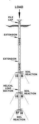
This drawing shows the tubular pile configuration for the 190 *ECP Torque Anchor*<sup>™</sup> helical screw pile that were installed.
