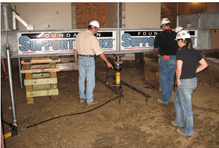
Load test set up prior to installation of production piles
