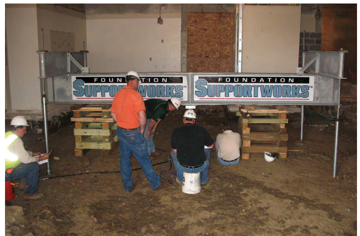
Load test completed and design capacities confirmed
